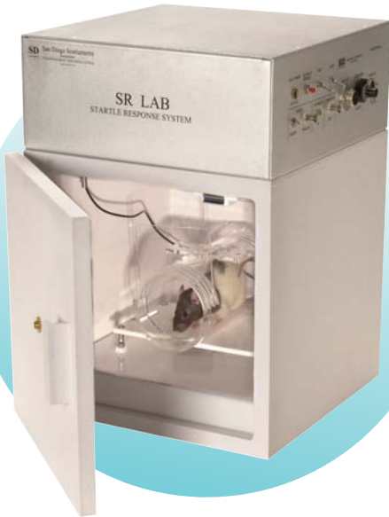
Complete SR-LAB test station with animal enclosure installed in the isolation cabinet
